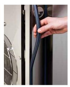
PLUG IN CONTINUOUS OVEN DOOR SEAL
